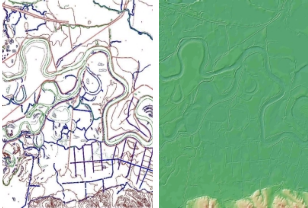
Picture 8. Left - Data from which the DEM is generated; Right - DEM presented by hipsoscale
